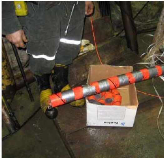
Figure 8 Eight Pentolite boosters (Preece, 2011)
